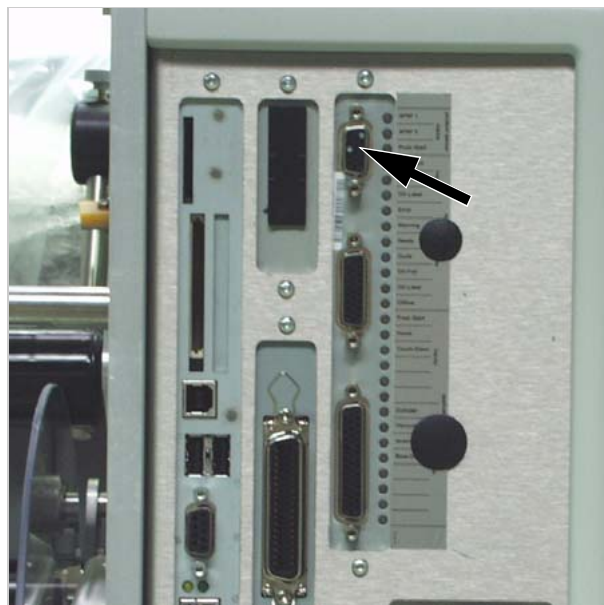
[20] Product sensor connection (arrow).
