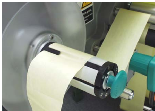
[49] Fastening the backing paper to the rewinder.
