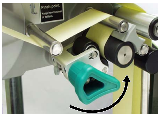
[48] Close the pressure roller.
