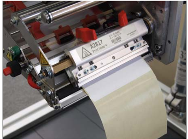
[35] Peel the labels off on a length of 50 cm.
