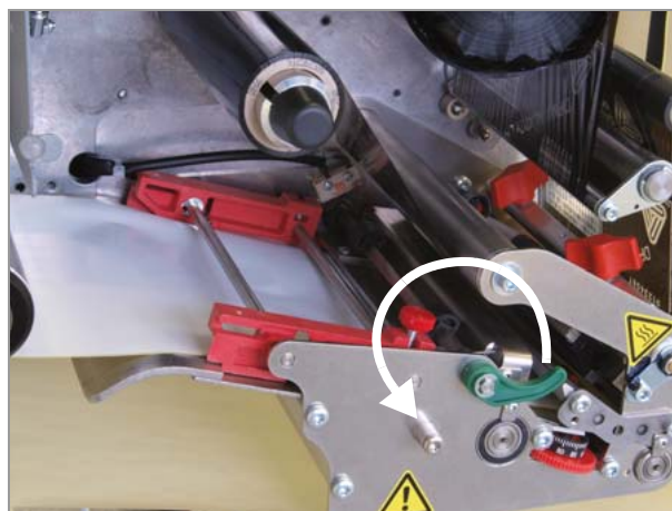
[41] Shut the lever for the pressure roller.
