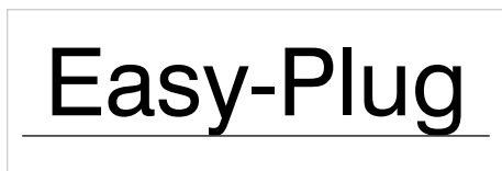
Fig. 7: Base line of a text. Even if the text has no descenders (as the y and the g in the example text), the base line lies a certain distance below the text.
