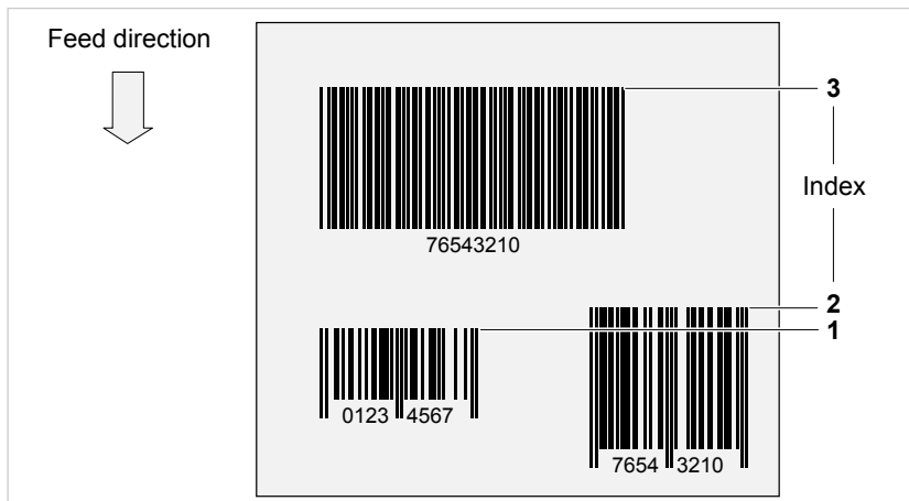
Fig. 13: The indexing of the bar codes is done in the order of the bar code top edges on the label in feed direction.
