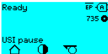
Fig. 52: Example of a USI status message (The XPM 94x doesn’t show the icon).
