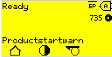
Fig. 51: Example of an USI warning: “Productstartwarn” (The XPM 94x doesn’t show the icon).
