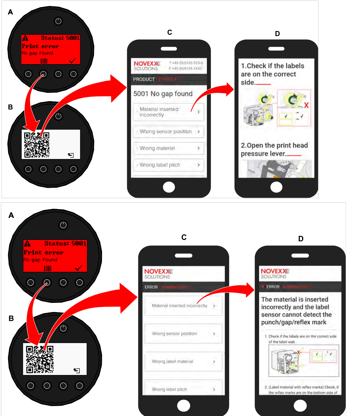
Fig. 53: If the error message has a barcode symbol (A), a QR code (B) can be used to call up troubleshooting instructions (C) on the smartphone.
