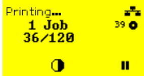
Fig. 43: Ribbon warning during a print job: yellow background, the ribbon icon flashes.
