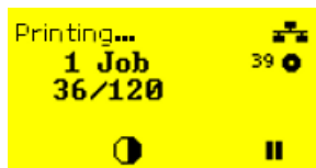
[58] Foil warning during a printjob: yellow background, the ribbon icon flashes.
