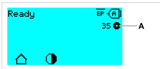
Fig. 44: Display of the remaining ribbon length (A, here: 35 m).
