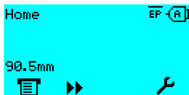
Fig. 41: Display of the measured label pitch.
