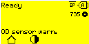
Fig. 55: Example of an USI warning: “OD sensor warn.”.
