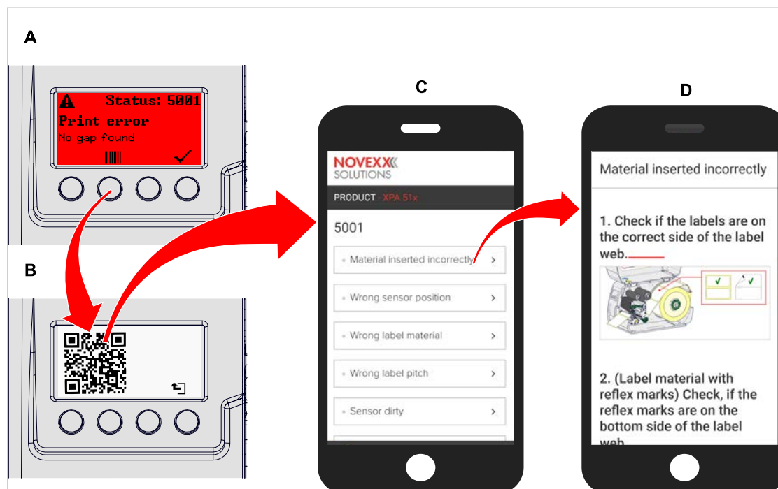
Fig. 57: If the error message has a barcode symbol (A), a QR code (B) can be used to call up troubleshooting instructions (C) on the smartphone.
