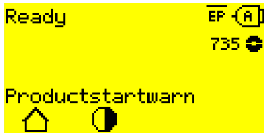
Fig. 55: Example of an USI warning: “Productstartwarn” .
