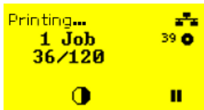
Fig. 49: Ribbon warning during a print job: yellow background, the ribbon icon flashes.
