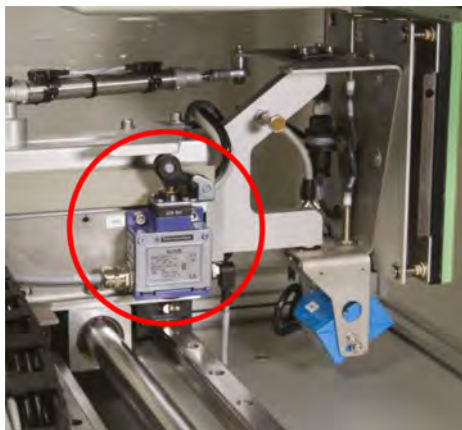
Fig. 21: Additional home position switch in the XPU.
