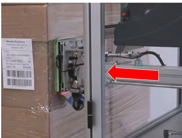
Fig. 8: The applicator presses the second label onto the side of the palett.
