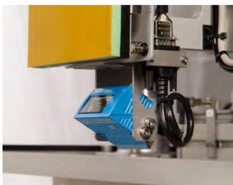
Fig. 18: The scanner option is mounted underneath the applicator pressure plate.
