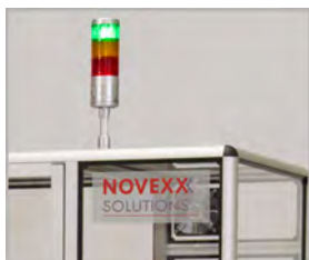
Fig. 36: The signal beacon on the cabin of the XPU lights green, yellow or red.
