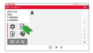
Select the desired label, choosing it from the disk [flash CPU disk C] or from disks [A/B] (USB memory stick).
