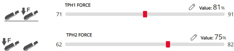
Figure 74: TPH force parameters for XTO22i.nn models
