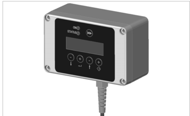
[531]External operator panel (Article number: A7474)
