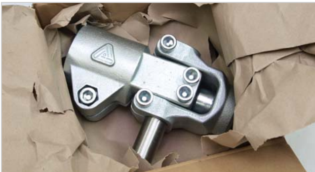
[465] State of delivery of the head joint brackets.
