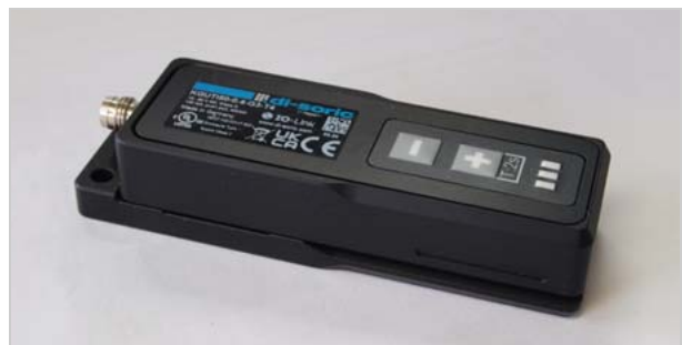
[28] Capacitive label sensor from di-soric KGUTI50 0.4-G3-T4
