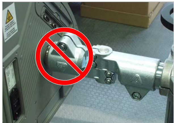
[7] Wrongly mounted head joint assembly. The clamp on the machine-side of the joint is pointing upwards!
