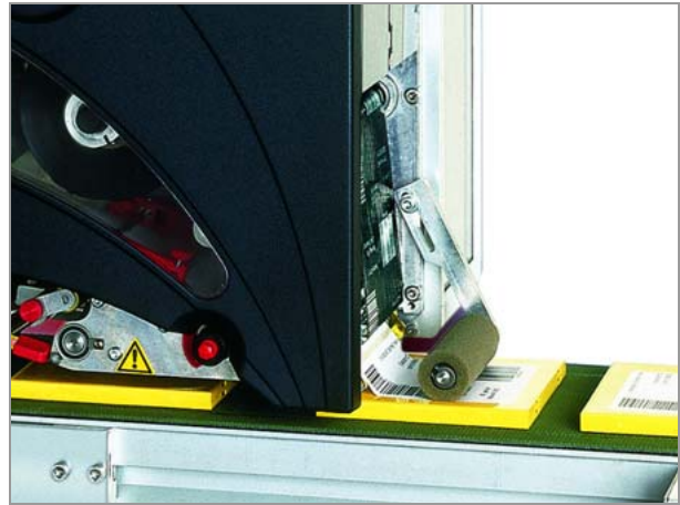
[4] Application example of the pressure roller.
