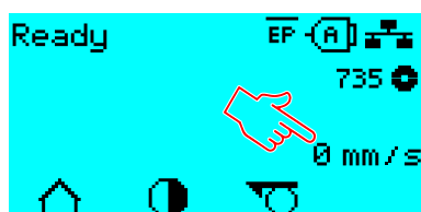
Fig. 54: The conveyor speed is displayed on the operating panel in APSF mode (with the unit set in the System > Speed unit parameter)
