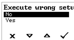
Fig. 50: Warning, if a wrong setup file was selected. The first line contains a scrolling text which shows a warning and afterwards the relevant file name. The answer in most cases should be "No".
