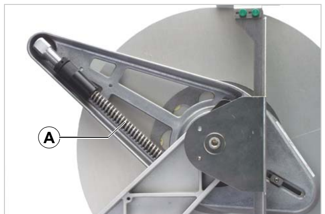
[50] Restoring spring (A) at the unwinder dancer arm.
