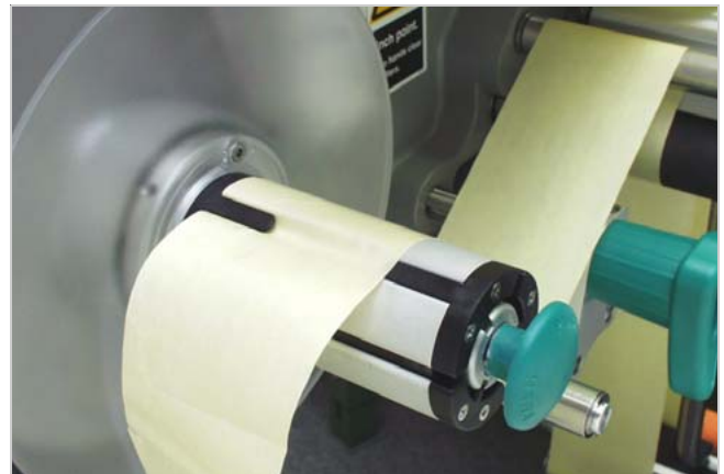
[45] Fastening the backing paper to the rewinder.
