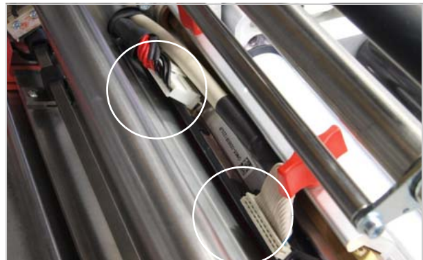
[101] Lay the connection cable so that it does not touch the ribbon.
