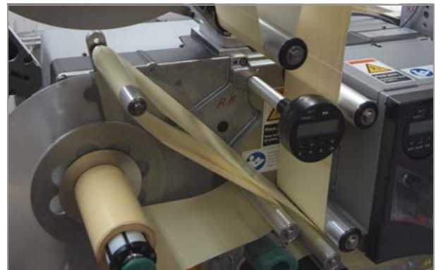
[62] Guide the backing paper around the dancer lever and deflection roller.
