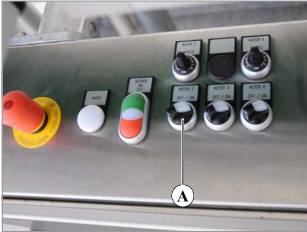
[5] ON/OFF switch (A) on the switch cabinet of the motor controller (Example: NOVEXX Solutions, AMC Series).
