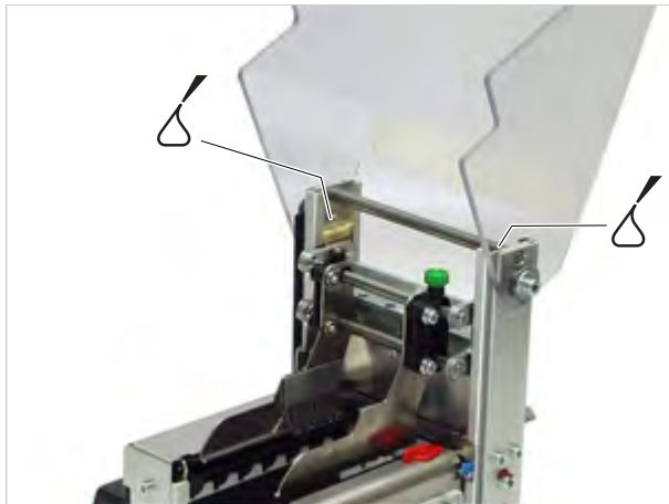
Fig. 6: Guides of the cutter slide.
