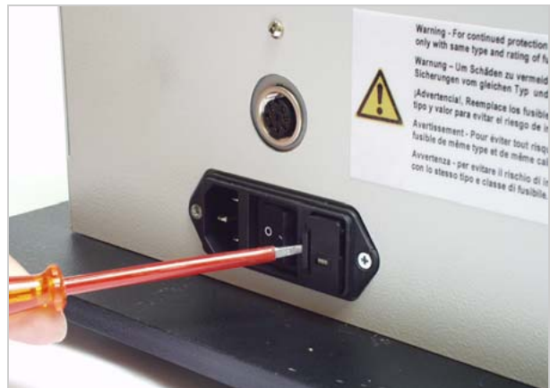
[10] Open the fuse insert latch with a screwdriver.
