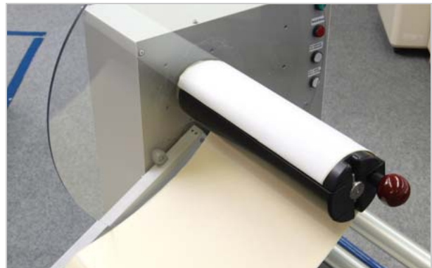
[5] (3" / 4") Feed the material end into the groove in the rewinding mandrel.
