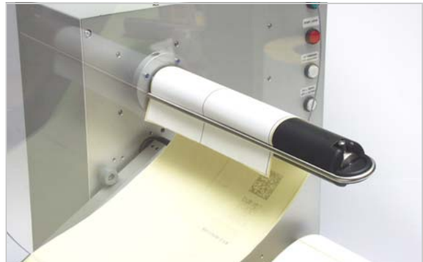
[4] (1,5") Securing the end of the material under the lock clamp.
