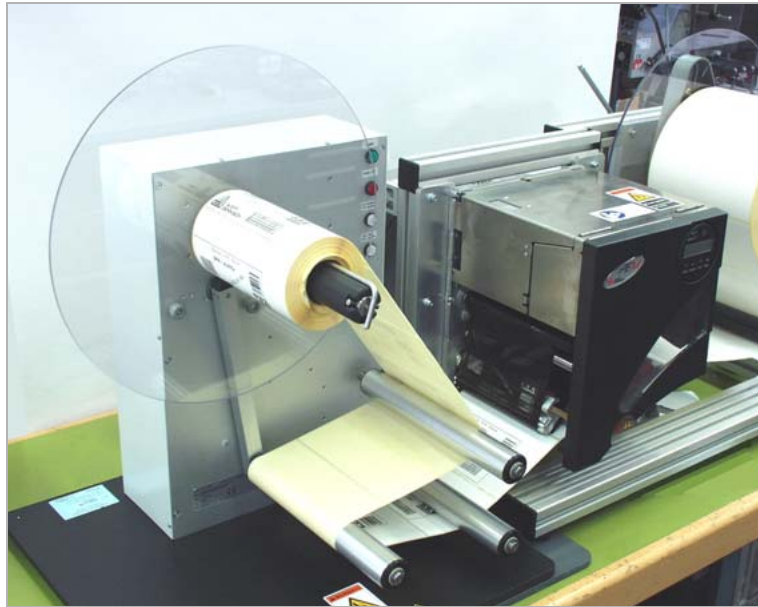
[1] The U-RX in a typical application: Rewinding label material after it was printed with a PEM printing module.
