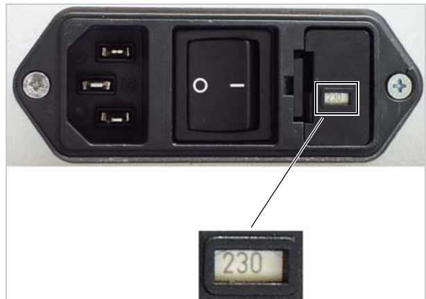
[1] Check the mains voltage set for the U-RX on the power socket of the unit (shown here as 230 V).
