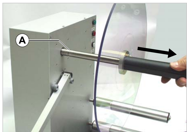
[9] Pulling out the rewriter mandrel
