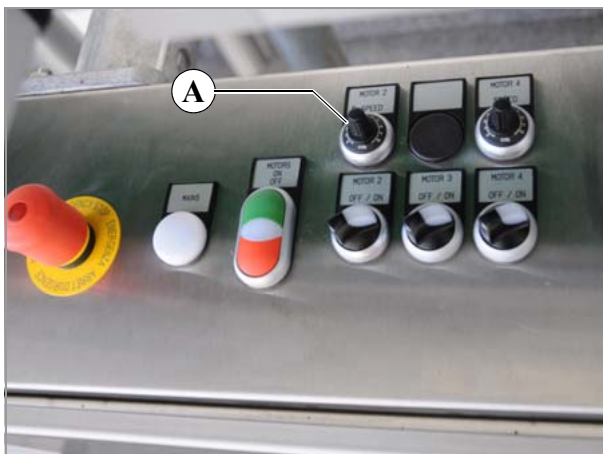
[15] Potentiometer (A) on the switch cabinet of the motor controller (Example: NOVEXX Solutions, AMC Series).
