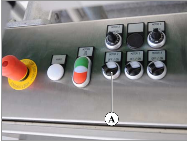
[6] ON/OFF switch (A) on the switch cabinet of the motor controller (Example: NOVEXX Solutions, AMC Series).
