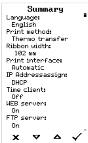
Fig. 35: Summary of the settings done by the wizard (Example, merged by image processing, in fact it must be scrolled to see all lines).
