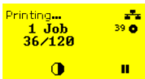
Fig. 46: Ribbon warning during a print job: yellow background, the ribbon icon flashes.
