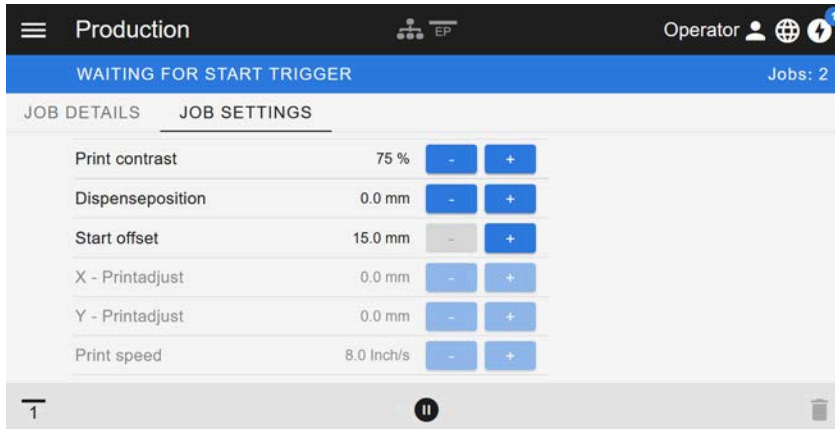
Fig. 21: View “Job Settings” of a print job in the web panel. Settings not accessible with the active role (here: “Operator”) are greyed out. The other settings can be changed by clicking on “+” or “-”.
