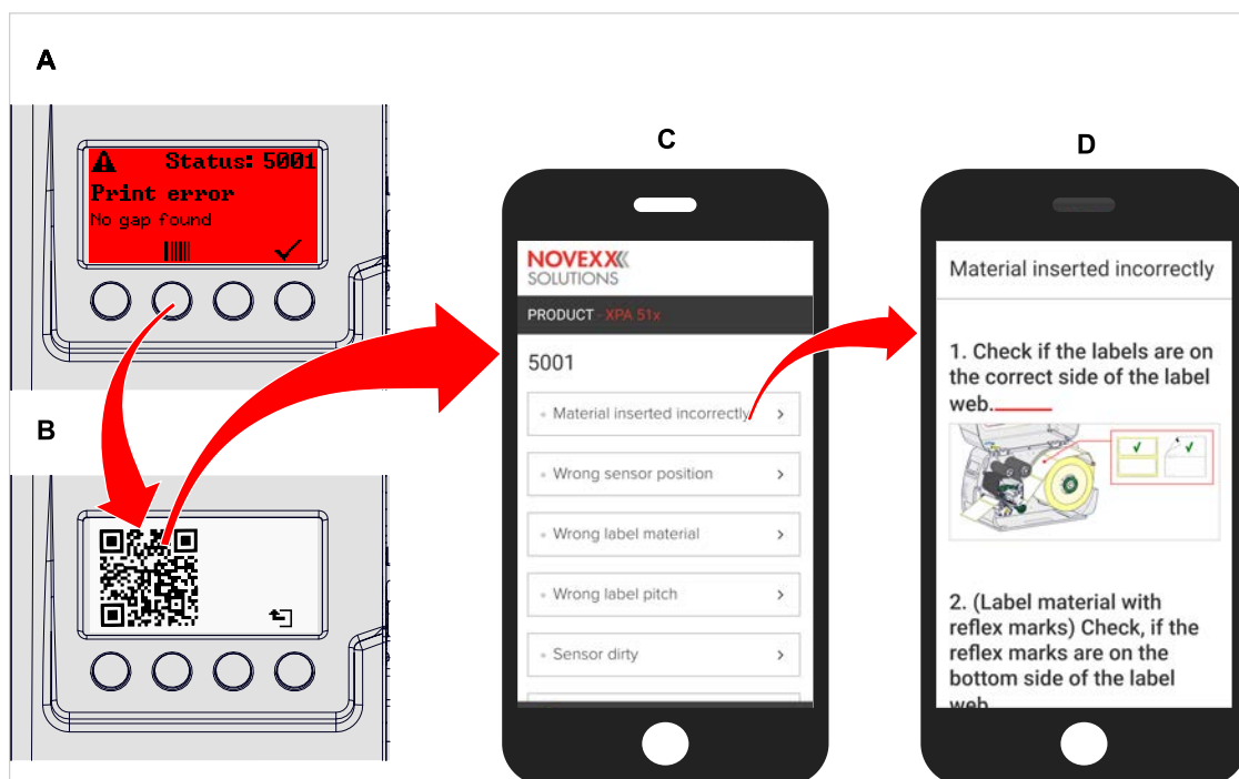
Fig. 58: If the error message has a barcode symbol (A), a QR code (B) can be used to call up troubleshooting instructions (C) on the smartphone.
