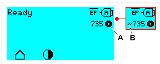
Fig. 44: Display of the remaining ribbon length (A, here: 35 m).
