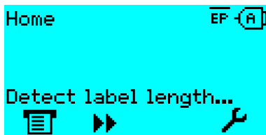
Fig. 47: The label pitch is being measured.
