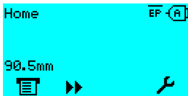
Fig. 48: Display of the measured label pitch.
