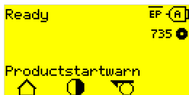
Fig. 70: Example of an USI warning: “Productstartwarn” .
