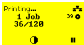
Fig. 61: Ribbon warning during a print job: yellow background, the ribbon icon flashes.
