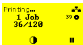
Fig. 71: Ribbon warning during a print job: The background is yellow, the ribbon icon flashes.
