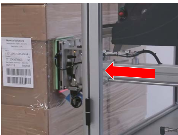
Fig. 7: The applicator presses the second label onto the side of the palett.
