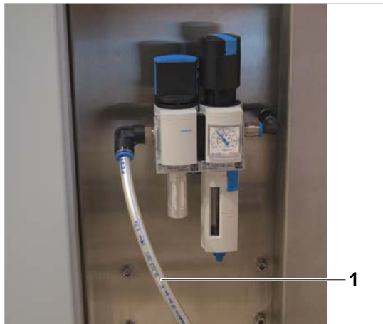
Fig. 14: Connect a "PUN 10 x 1,5" pneumatic hose to the service unit at the XPU (1) and to the compressed air supply.
