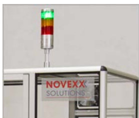
Fig. 35: The signal beacon on the cabin of the XPU lights green, yellow or red.
