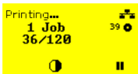
Fig. 28: Ribbon warning during a print job: yellow background, the ribbon icon flashes.
