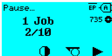
Fig. 34: Stopped print job. Press key 4 to continue printing.
