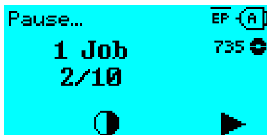
Fig. 52: Stopped print job. Press key 4 to continue printing.
