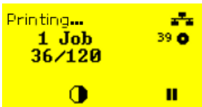
Fig. 56: Ribbon warning during a print job: The background is yellow, the ribbon icon flashes.
