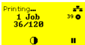
Fig. 46: Ribbon warning during a print job: yellow background, the ribbon icon flashes.
